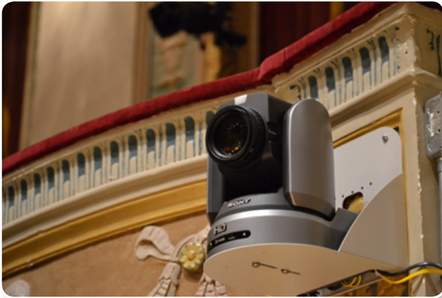
One of the six robotic Sony HD cameras affixed to the walls of Orchestra Hall.
